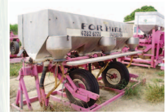
Above: Horstine Microband metering units on a large-scale suSCon Maxi applicator on a dual-purpose toolbar. Important features are the ground drive and depth wheel; straight drop to row; and backward-sloping, row-centred tine to deflect cane shoots and direct the granule band to the row centre. Granules are covered in a separate operation.
