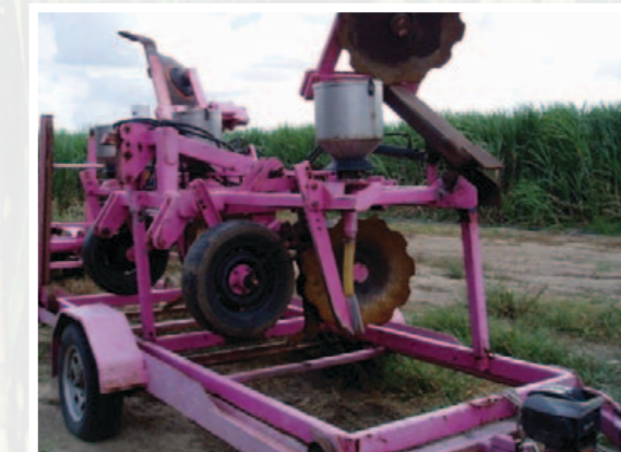
Above: Microband granule applicators fitted to a cultivator - designed to apply suSCon Maxi and to fill-in plant cane in one pass. Important features are the stout tine leg to deflect cane shoots and direct the granule band to the row centre; applicators sitting directly over the row to keep granules flowing through the tubes; and discs and tines to fill-in and start hill-up.
