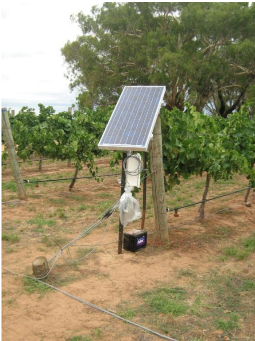
Date logger set up last season in Victoria to monitor water use showed reduced water stress in marsanne vines treated with Parasol sunshield.
